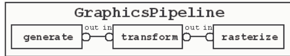
Fig. 2. The GraphicsPipeline is a pipeline made up of three subcomponents: the generate , the transform and the rasterize subcomponents.
