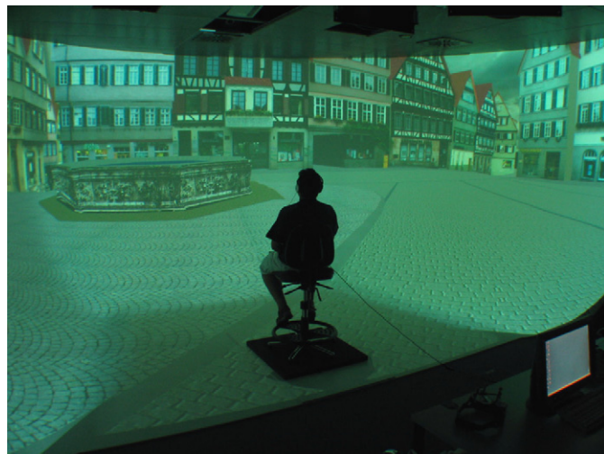
Fig. 1. The Pano Lab: semi-spherical projection screen with 220 horizontal by 165 vertical field of view (FOV).
