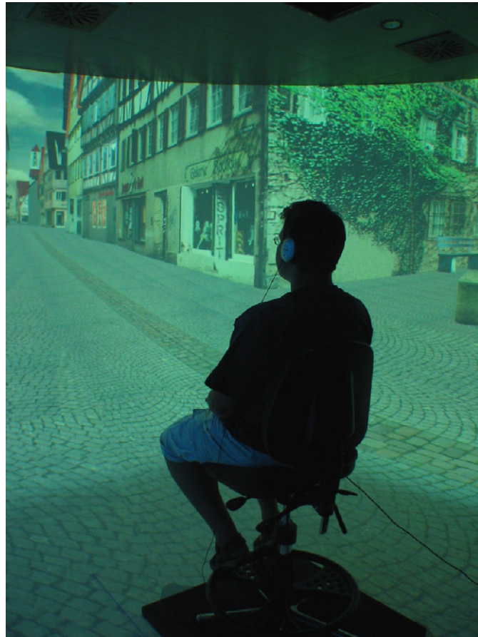
Fig. 5. Pano Lab with three-dimensional virtual town used for linear vection. The participant is always sitting in the same way and the only difference between the floor and no floor condition is that the floor projector is turned off in the latter case.
