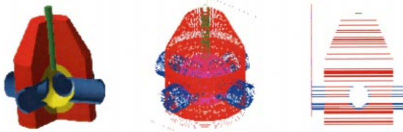
Fig. 14 Adaptive slicing of heterogeneous objects
