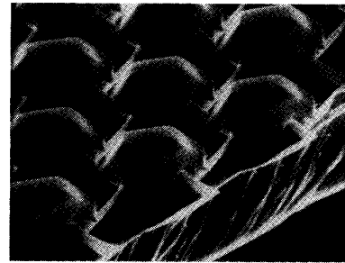
Fig. 2. Electron micrograph of micromechanical fastening structures.
