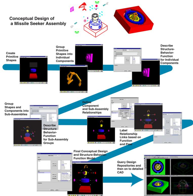
**Fig. 3.** The conceptual design process of the missile seeker within CUP, from component design to functional description to final conceptual assembly. This conceptual design then becomes the basis for detailed CAD.
