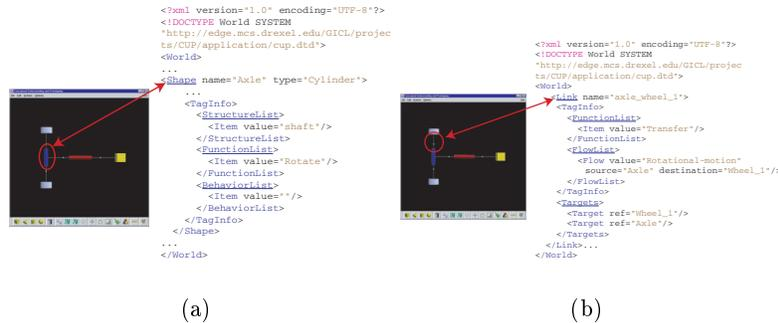
**Fig. 2.** Snippets of XML code from an assembly modeled in CUP (specifically, a simplified drive train).
