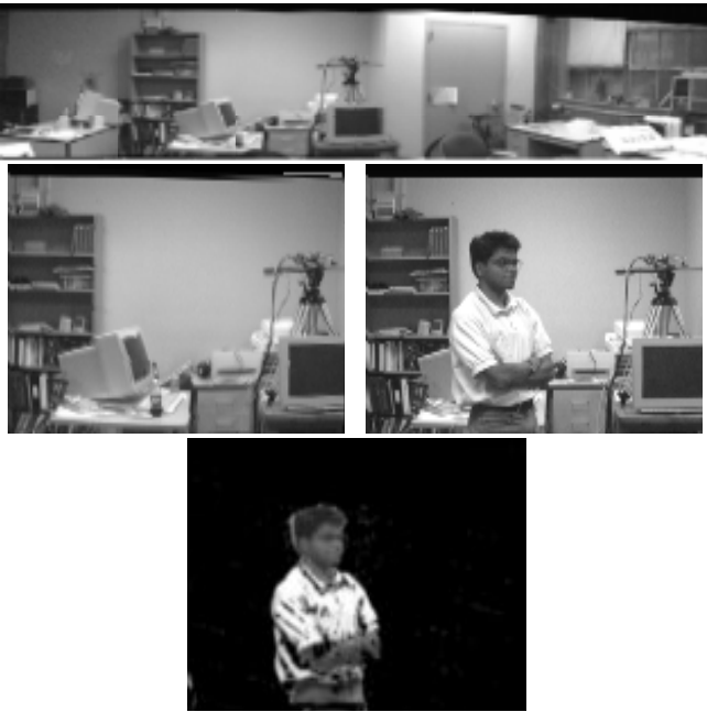
Fig 3. The top image shows a panoramic background image mosaic constructed using a set of background images. The next row shows two images where the right image is a frame captured for the current pan and tilt position and the left image is the corresponding background image indexed from the mosaic. The bottom image shows the segmented foreground object.
