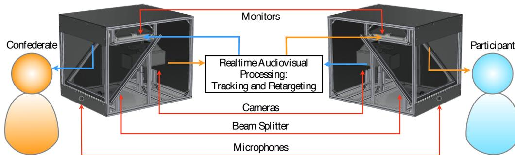
Figure 2. Diagram of telecommunications system.
