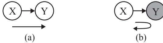
Figure 9. Boundary conditions. (a) If Y is unobserved, the ball leaves the graph. (b) If Y is observed, the ball bounces back to X .
