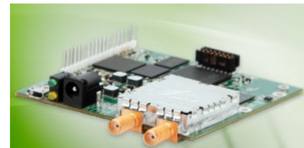
UWB range sensing module: accuracy 2cm (TimeDomain)
