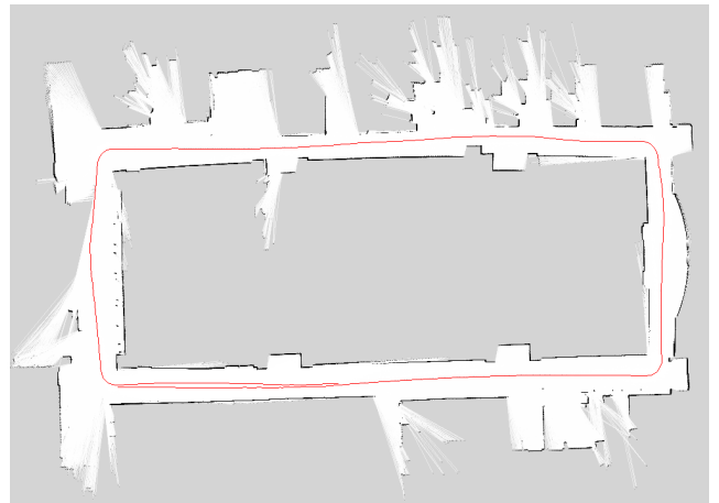
Fig. 3. Evidence grid plot after loop closing (TSRB). Better local alignment of scans can be achieved by other methods, but is not done here to show the result based on sparse features only. The trajectory covers approximately 40 meters by 15 meters.
