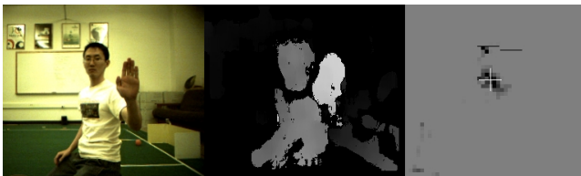
Figure 5: Stereo vision: color image from stereo image pair (left), calculated depth map (center), projected top-down occupancy map (right).
