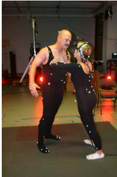
Figure 3.10: MMM capture session. The red lights are the real light Vicon cameras, the woman is wearing a transmitter on her back, an eye-tracker is fixed on her head.
