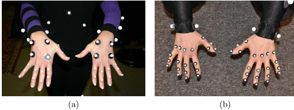
Figure 3.8: Marker sets of the hands used for the captures: (a) MMM; (b) narration. The differences between the marker sets are the placement and number of the markers on the thumb and the dorsal surface.
