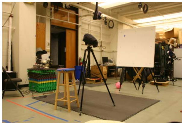
Figure 3.15: Calibration setup. The subject sits down on the bar stool and puts his or her chin on the tripod to stabilize the head. The nine points that need to be fixated form a grid on the white board.
