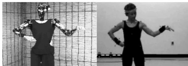
**Figure 1:** The Sarcos humanoid robot at ATR (DB) tracking motion capture data of a human actor.
