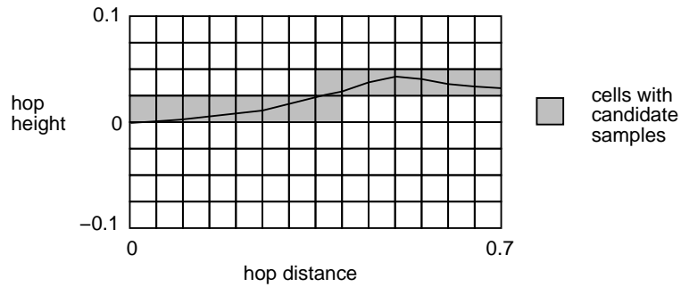
Figure 4: Using the terrain to restrict the candidate motions
