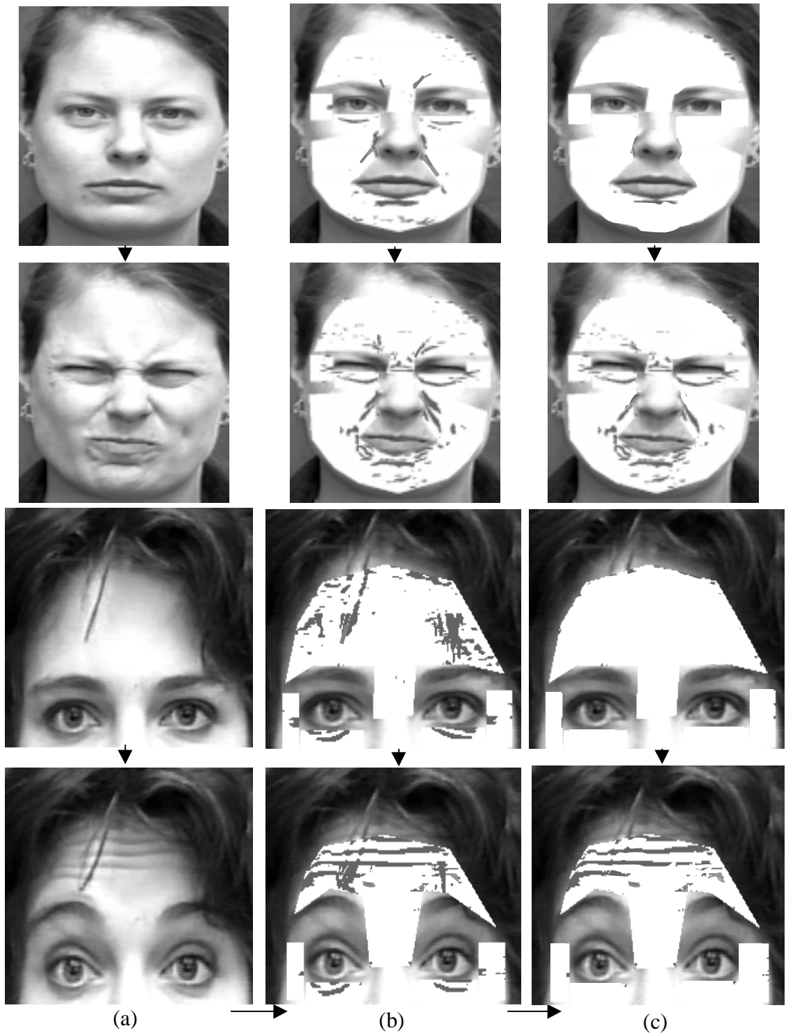
Figure 35 (a) Original gray value images. (b) High gradient component (furrow) detection in the spatial domain. (c) High gradient component analysis in the spatio-temporal domain.
