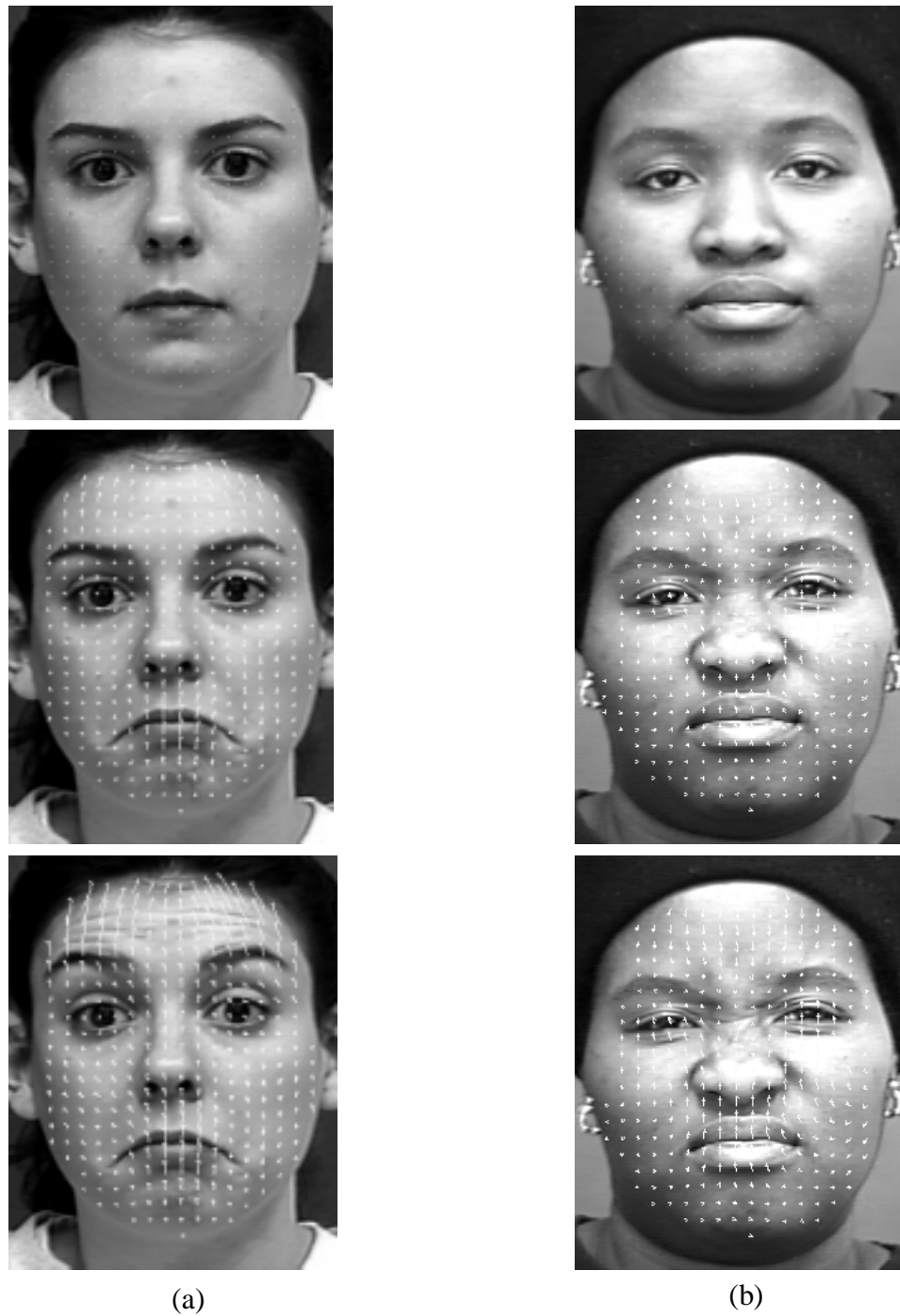
Figure 24 Good tracking performance of using the wavelet-based dense flow for (a) furrow discontinuities at the forehead and chin regions, and (b) textureless regions with reflections at the forehead and cheek.
