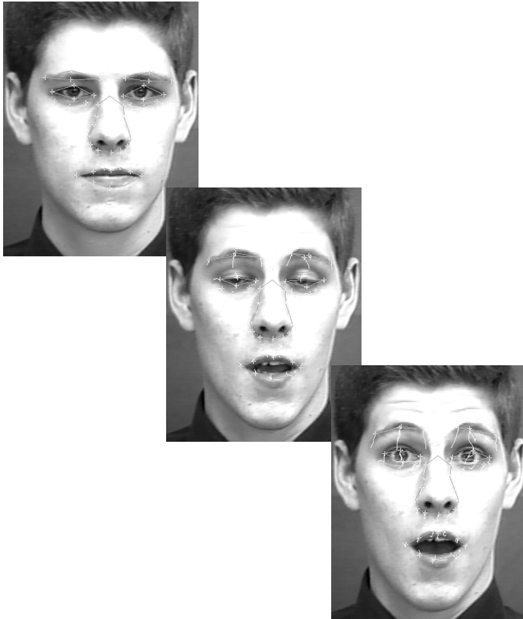
Figure 12 Feature point tracking excluding the pyramid method: it is sensitive to subtle motion such as eye blinking, but it loses tracking for large motion such as mouth opening and suddenly raising eye brows. Lines trailing along feature points (marked by a cross '+') denote their movements across image frames in the sequence.
