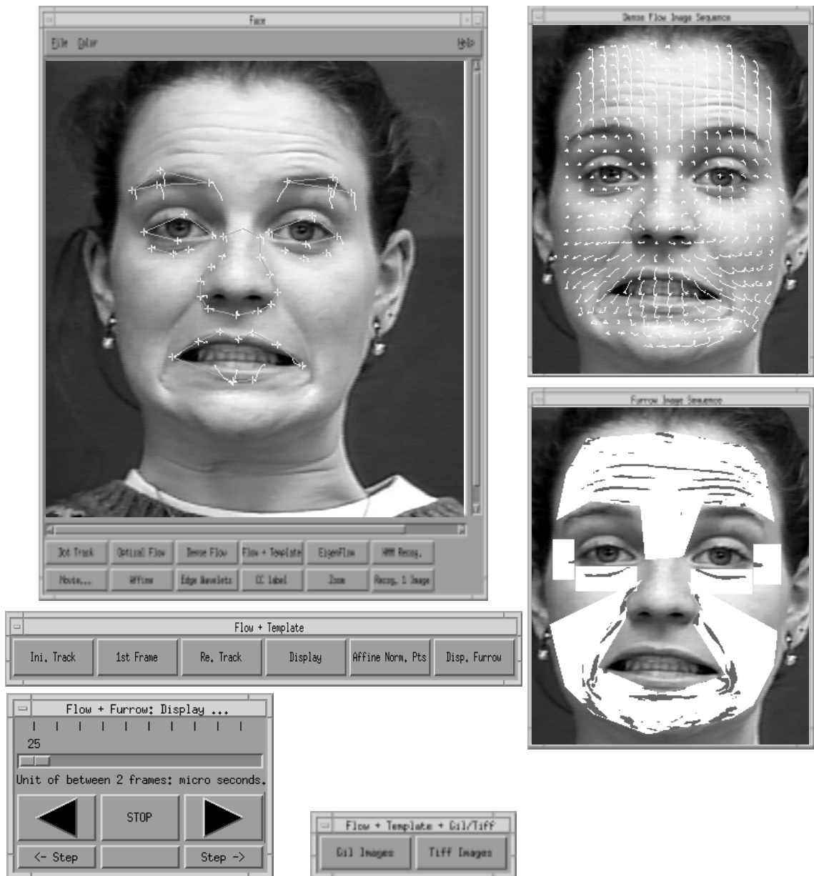
Figure 2 The user interface created by programming in C, Motif, X Toolkit and Xlib.
