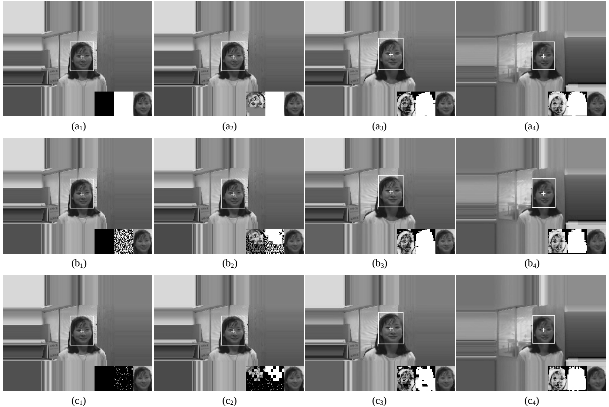
Fig. 13. Demonstration of the error-correction capability possessed by the CAPOA algorithm. The corruption degree of the initial outlier map increases from the top row to the bottom row. The four columns from left to right show frames 1, 2, 8, 16 of the sequence seq_mb , respectively. The tracked target (ROI) is indicated by a white rectangle with a cross at the center. In the lower right corner of each image, the current Kalman gain, the current template mask and the current template are displayed from left to right. The Kalman gain is displayed on a scale of 0 to 1, where brighter pixels indicate higher Kalman gains. In the template mask, the masked portion is indicated in black.
