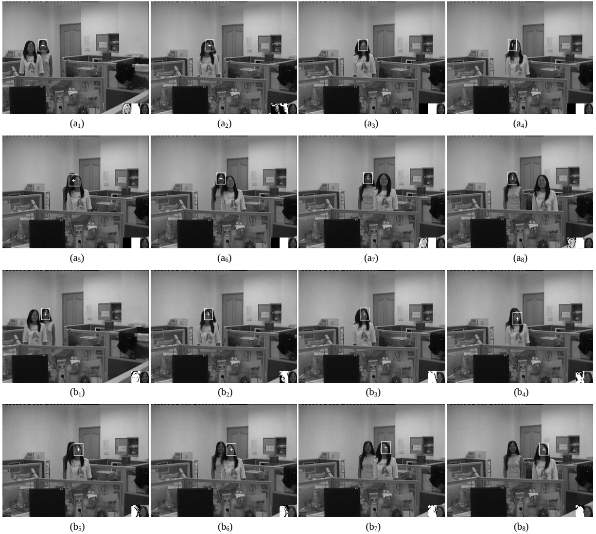
Fig. 8. Illustration of the tracking process of our proposed tracker and the RAF-based tracker under a short-term complete occlusion at frames 53, 64, 68, 71, 74, 77, 82, and 90. The sequence under test is shot by us. The tracked target (ROI) is indicated by a white rectangle with a cross at the center. (a 1 )-(a 8 ) The tracking process of our proposed tracker, where the lower right corner of each image is overlapped from left to right by the current Kalman gain, the current template mask and the current template. The Kalman gain is displayed on a scale of 0 to 1, where brighter pixels indicate higher Kalman gains. In the template mask, the masked portion is indicated in black. (b 1 )-(b 8 ) The tracking process of the RAF-based tracker, where the lower right corner of each image is overlapped from left to right by the current outlier situations of the template and the current template. Outlier pixels are indicated in black.
