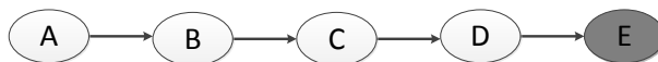
Figure 4: Bayesian network of five random variables A, B, C, D, E where E is observed.
