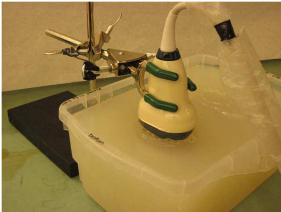
Figure 3.6: For ultrasound acquisition, the 3D curvilinear probe is clamped in place above the phantom.
