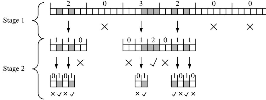
Figure 3: Illustration of the sensor probing algorithm.
