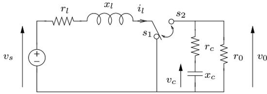
Figure 3: Boost DC-DC converter.
