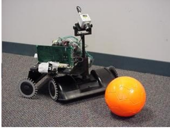
Figure 7: The first minnow robot tracking a soccer ball.
