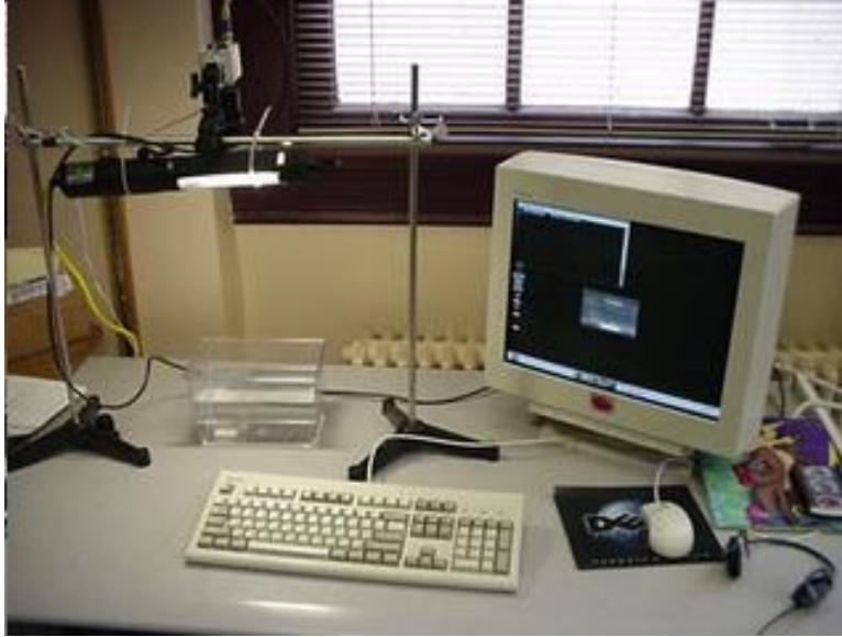
Figure 9: The experimental apparatus set up to track fish.
