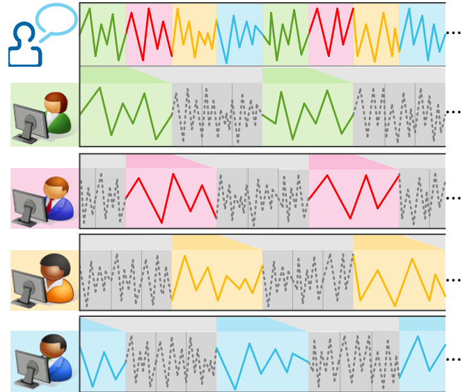
Figure 1. TimeWarp forwards different “warped” versions of the audio to each worker. Workers hear a slowed down version of the content they are supposed to caption, while they hear the rest sped up. This increases the quality of workers’ output by asking them to complete an easier task without losing context. The start of each slowed segment is aligned with the original audio, allowing the crowd to collectively caption in real time.
