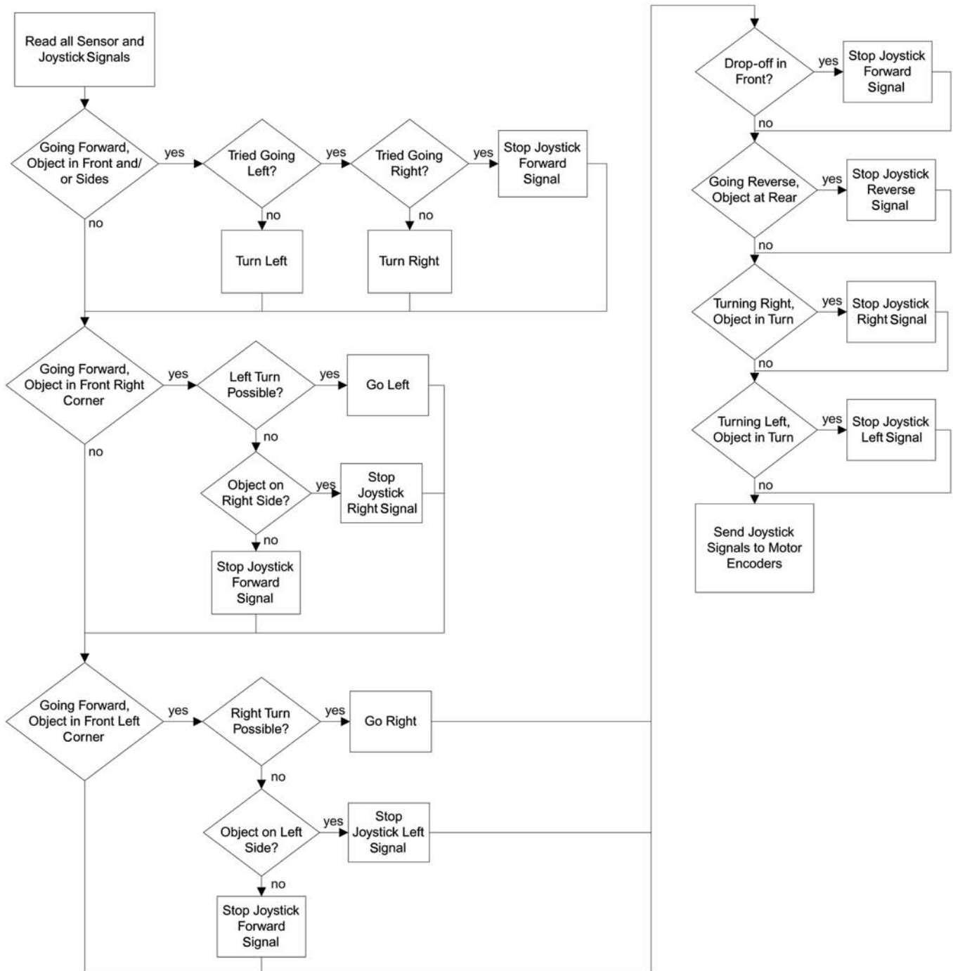
Figure 4. Flowchart of navigation assistance algorithm used during reliability testing.
