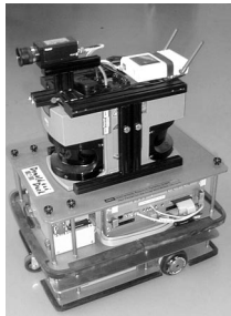
Figure 5: The fully autonomous robot Donald Duck. Its controller consists of a VME standard backplane with a Motorola PowerPC 604 microprocessor clocked at 300 Mhz running XO/2. Among its peripheral devices, the most important are the wheel encoders, a 360° laser range finder and a grey-level CCD camera (not used here).
