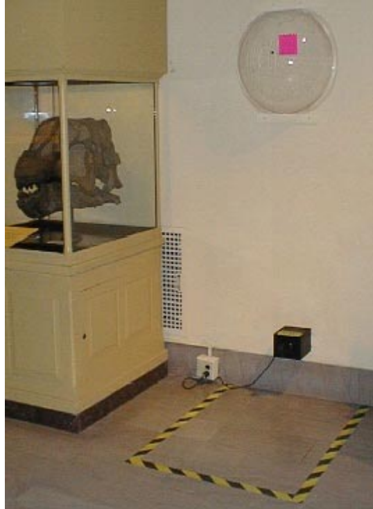
Figure 9: Sage’s recharging outlet and, above it, the 3D marker used during docking. In this case, the 3D marker consists of an acrylic hemisphere with a black square painted on it, encasing a flat pink 2D marker.
