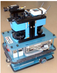
Fig. 6. The fully autonomous robot Donald Duck. Its controller consists of a VME standard backplane with a Motorola PowerPC 604 microprocessor clocked at 300 Mhz running XO/2. Among its peripheral devices, the most important are the wheel encoders, a 360° laser range finder and a grey-level CCD camera.
