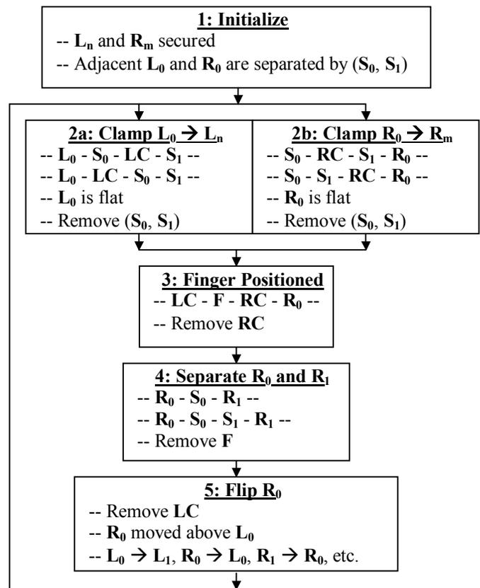
Figure 2: Flowchart of page flip cycle
