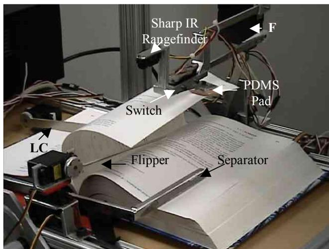
Figure 6: Current prototype of the page manipulating robot. Clockwise in the plane of the book from the bottom right corner the arms are: the separator, the flipper, LC and F.
