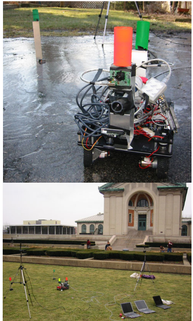
Figure 1. Robots On Ice, In the Grass. Note the tripods for the robot tracking system and the laptop computers used to record video.
