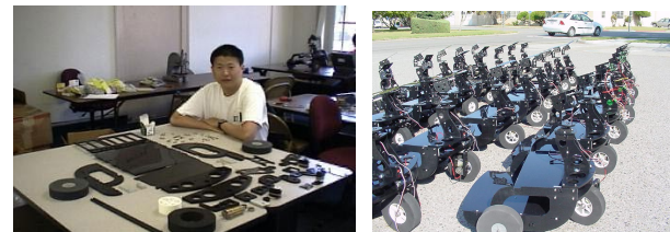
Figure 3: The unassembled components of one Trikebot; 30 assembled Trikebots (right)
