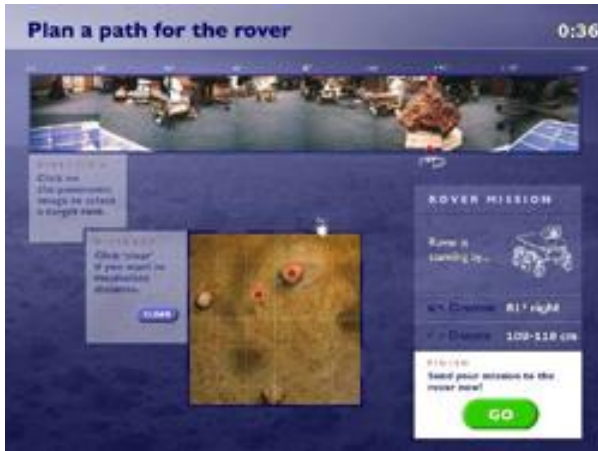
Fig. 3. The mission generation screen of the PER's kiosk interface.
