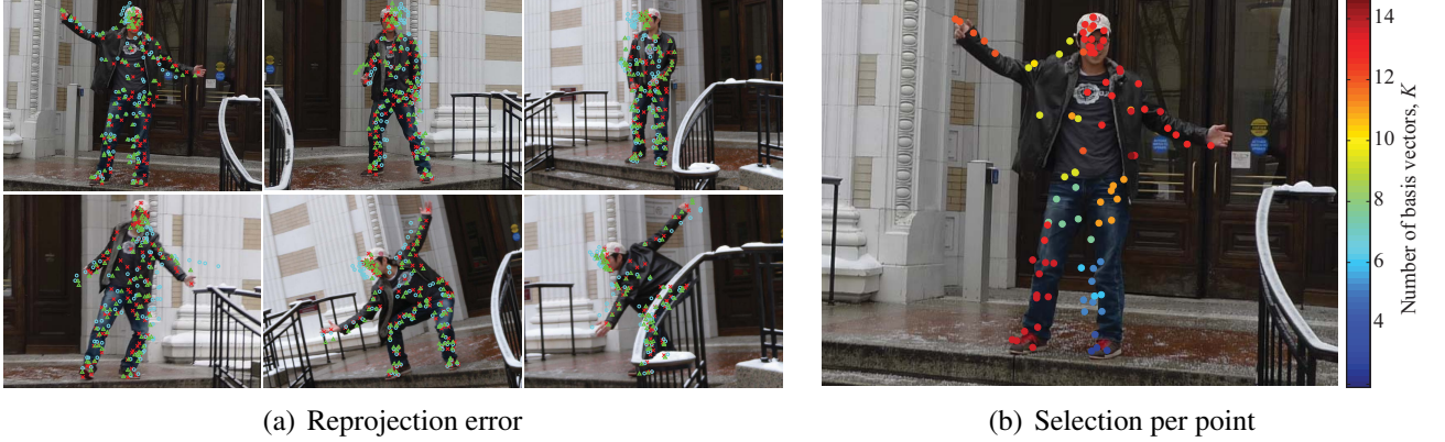
Figure 5.13: Reprojections of trajectories from manually selected K and automatically selected K_i are shown for the dance scene. (a) Red cross: measurement, cyan circle: manually selected K , and green triangle: automatically and individually selected K_i . Trajectory from K_i has smaller reprojection error. Average reprojections for K and K_i are 11.55 and 6.47, respectively. (b) The number of basis vectors per point is color-coded. The points on the hands require many basis vectors while the points on the left leg which barely move requires few basis vectors.
