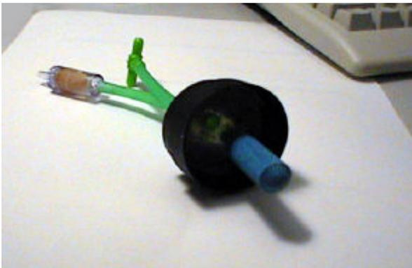
Figure 4. End Cap Assembly with Diffuser, Drain Hose, and Check Valve
