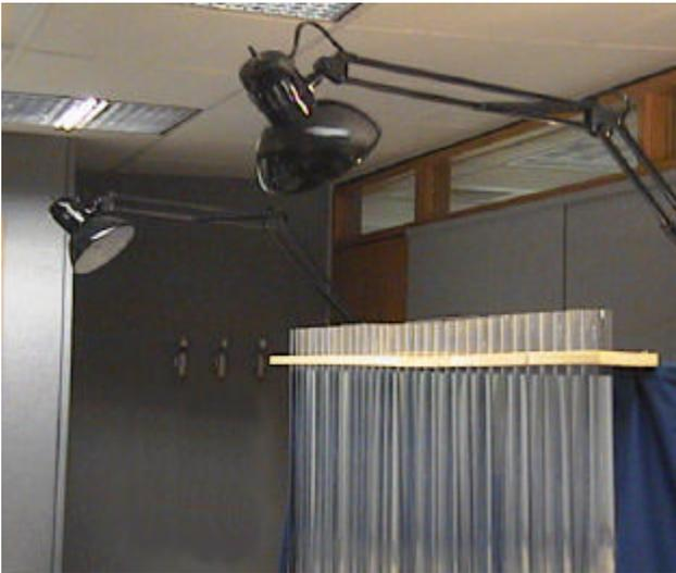
Figure 6. Placement of Lighting for High Contrast
