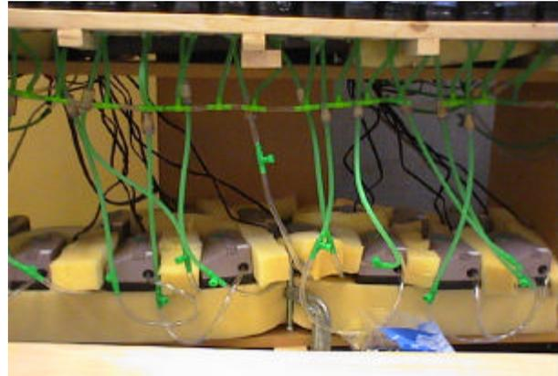
Figure 7. Sound Dampening Around Pumps
