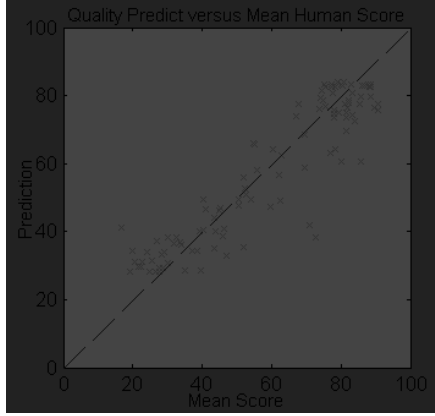
Fig. 2. Quality prediction versus mean human score for JPEG compressed images
