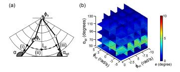
Fig. 2. Robust swing leg controller. (a) The swing controller reaches  $\alpha_{tgt}$  while ensuring ground clearance  $l_{clr}$ , and uses hip  $(\phi_h)$  and knee  $(\phi_k)$  angular data as sensory inputs. The knee controller follows a three-part control sequence (details in text). (b) The placement error  $e = |\alpha_{tgt} - \alpha_{td}|$  is shown for largely different initial angular velocities  $(\alpha_{td}$  is leg angle at touch down).
