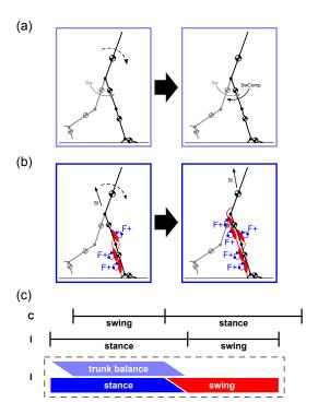
Fig. 3. Modifications made in the neurocontroller. Feedforward controllers are added to (a) the trunk balance control to compensate moments induced by the swing leg and (b) the stance control to compensate ground reaction forces transferred by the stance leg. In addition, the explicit swing initiation control required in the previous neuromuscular control is now removed (c).
