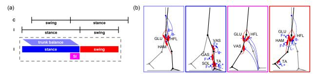
Fig. 1. The functional control groups of the previous neuromuscular model for human walking [19]. The control architecture is grouped into the control of trunk balance, stance, swing initiation (SI), and swing. The sequencing of the control groups and schematics of the active reflex pathways are shown in (a) and (b), respectively (color matched). In (a), I and C refer to the ipsilateral and contralateral leg.
