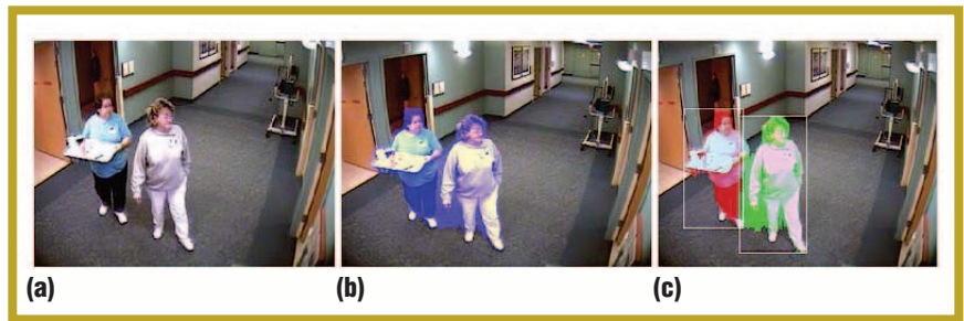
Figure 1. An example of using a mean-shift algorithm to split merged people: (a) the original video, (b) merged tracking, and (c) tracking a split with mean shift.
