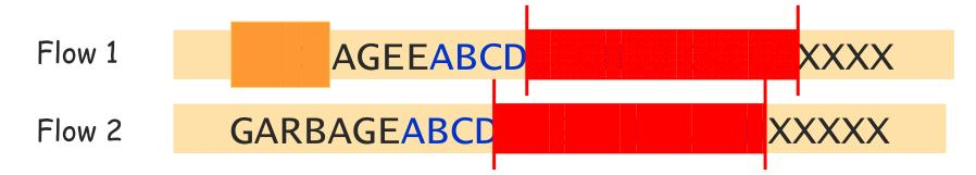
Breakmark = last 8 bits of fingerprint (ABCD)
