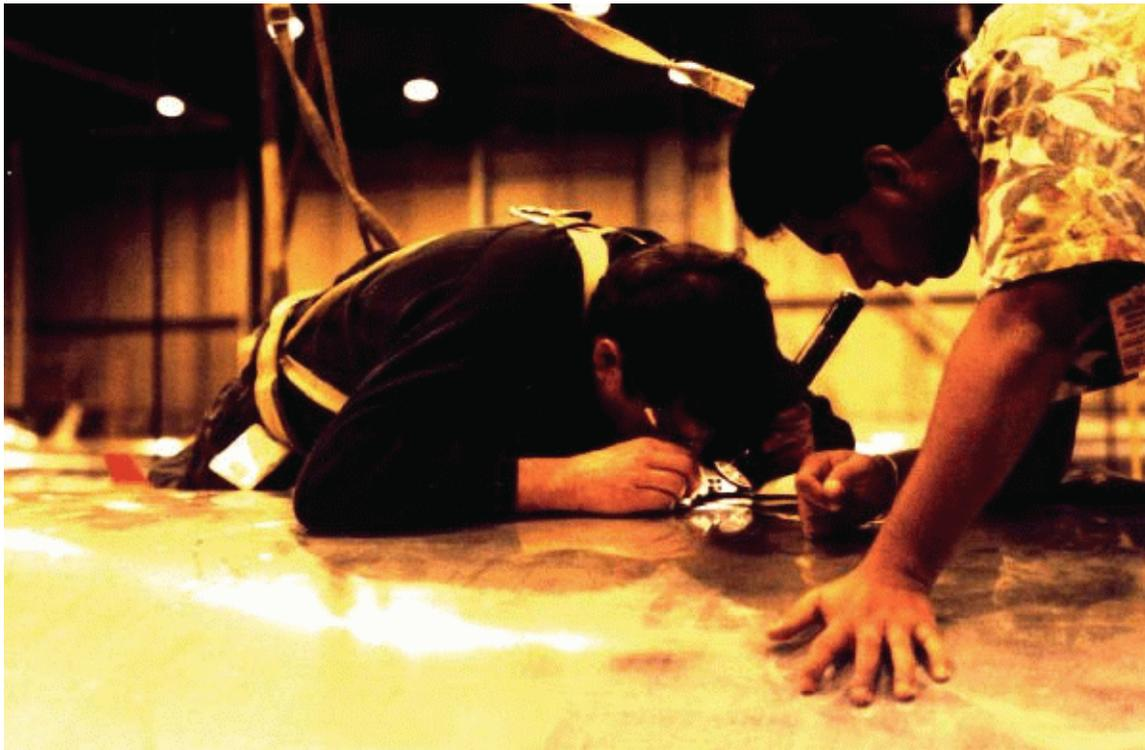
Figure 1: Aircraft inspector (with flashlight and 10x magnifier) and author P.G. inspecting the crown of a Boeing 737 airplane. Note safety harnesses.
