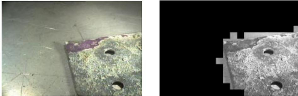
Figure 7: (left) Corrosion surrounding rivet holes in a disassembled lap joint. (right) output of the corrosion detection algorithm.
