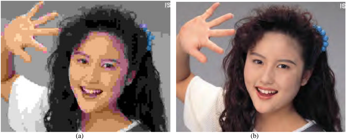
Fig. 20. Reconstructed images compressed at 0.125 bpp by means of (a) JPEG and (b) JPEG2000
