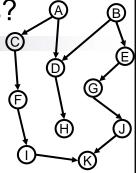
■ Theorem: If G₁ and G₂ have the same skeleton and V-structures, then G₁ and G₂ are I-equivalent
