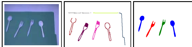
Figure 1. Contour extraction. Left: Raw image (poor white balance in the camera results in poor colour rendering). Middle: Contours extracted using pyramid segmentation. Right: Contours extracted using intensity thresholding. Our goal is to recognize different objects from the same class from the complete or partial outline of each object.
