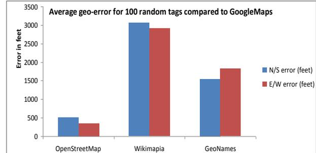
Figure 1 shows the N/S and E/W error in feet for 100 randomly-chosen tags for each of our Web 2.0 sites, and from our GeoNames gazetteer in comparison GoogleMaps
