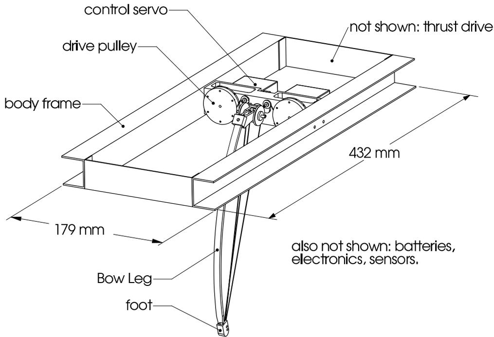
**Figure 1: Partial assembly diagram of the 3D Bow Leg Hopper.**
