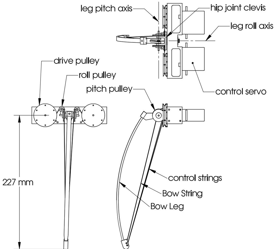
**Figure 2: Three views of 3D Bow Leg Hopper chassis.**
