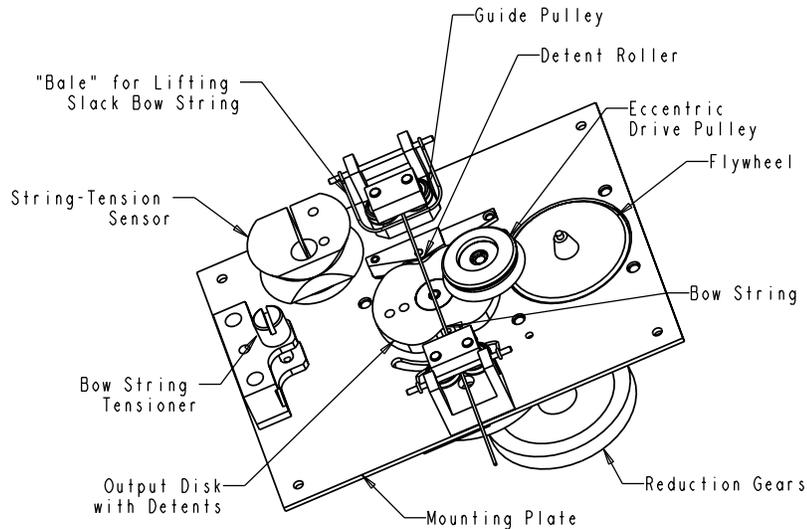
FLYWHEEL/CLUTCH RETRACT MECHANISM
