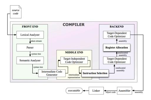
Figure 1: Structure of a typical compiler<sup>2</sup>
