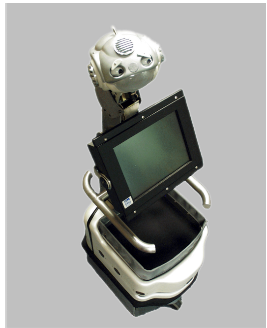
Figure 4: Pearl: A Mobile Robot Platform for the Autominder Cognitive Orthotic. Photo courtesy of Carnegie Mellon University.
