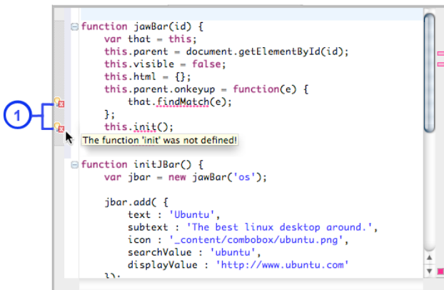
Figure 2: Euklas marks errors in the function jawBar() , which is the constructor of the enhanced combo-box, after Jamie pasted it into the target file.
