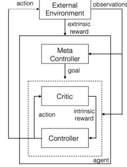
Figure 3. Control Sequence Describing the Meta-Controller and Controller Process
