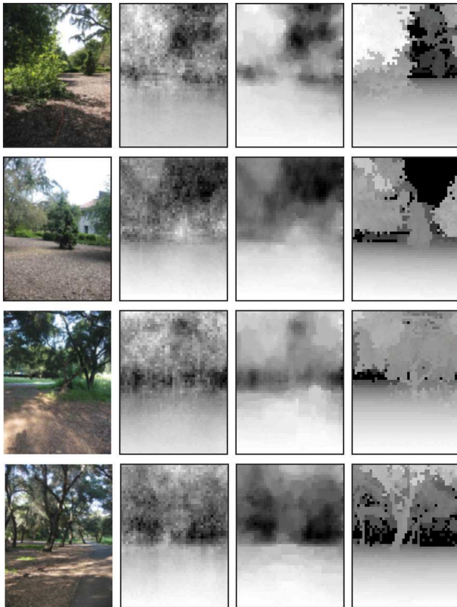
Figure 3: Linear regression and Markov random field estimates of depth given monocular images from the test set. The first column is the actual image, the second column is the linear regression estimate, the third column is the Markov random field estimate, and the fourth column is the true depth. Lighter is closer while darker is farther away. Note how the second term in the Markov random field smooths local depth estimates.
