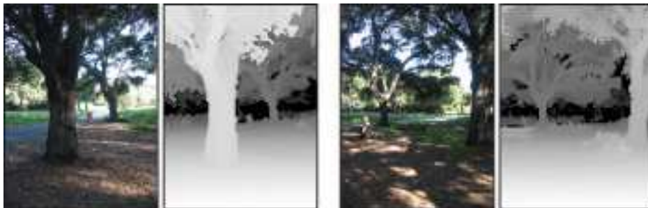
Figure 2: Examples of images and correlated depth maps. Lighter color indicates closer surfaces.
